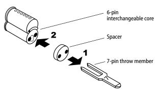
*Figure 1 — Sliding a spacer over a 7-pin throw member, then installing the throw member and spacer into the 6-pin core.*
