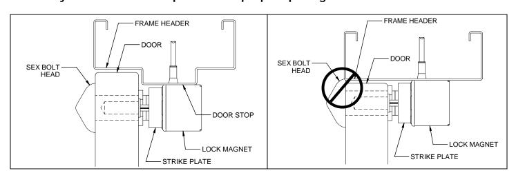
Figure 1 **Model 32 Installation**
