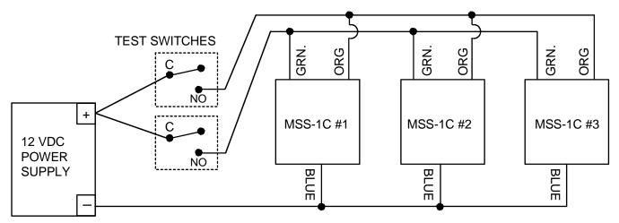
REMOTE TEST WIRING SHOWN WITH THREE MSS-1C SWITCHES. ANY NUMBER OF MSS SWITCHES CAN BE CONNECTED IN THIS WAY. NOTE THE TWO NORMALLY OPEN TEST SWITCHES. THEY SHOULD BE CLOSED ONE AT A TIME AND ALL MSS SWITCHES SHOULD GO INTO ALARM TWICE TO PASS THE TEST.
