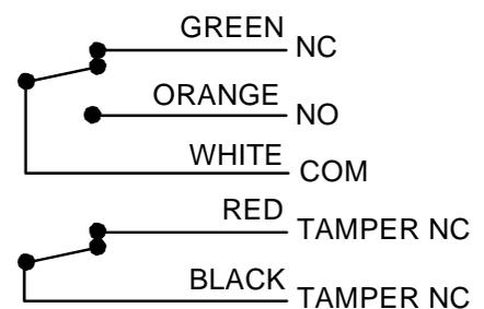
SCHEMATIC SHOWS SWITCH IN SECURE CONDITION WITH TAMPER FEATURE IN USE. CONTACTS WILL SWITCH WHEN SWITCH ALARMS OR TAMPER IS VIOLATED.
