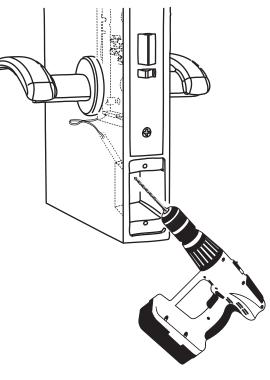
Metal B: Cut main pocket with rotary tool using a metal cutting wheel or a metal cutting saw
