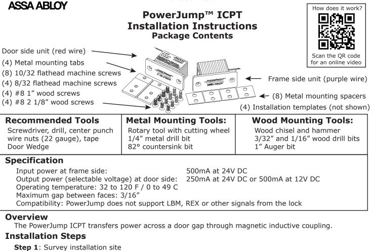
Unit may be installed on latch side, hinge side, top or bottom of door. Note the ICPT requires a depth of  $1 \frac{3}{8''}$  in the frame and  $1 \frac{5}{8''}$  in the door.
