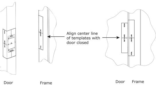
**PowerJump Mounted Dimensions** 0  $\odot$ 1 1/4" mounting tabs (2)  $\bigcirc$ Metal Mount Wood Mount Depth Face Face Frame Unit 1 3/8" 7/8″ 3/4" 1/8''1 1/4" μ  $\sim$  $\sim$ Door Unit 1 5/8" E Ý  $\bigcirc$ Hard Wood 3/32" x 3/4" deep Soft Wood 1/16" x 2" deep 0 0 1/4'' bit (4) places 82° countersink
