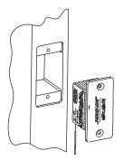
**Wood D:** Drill a wiring channel for connection to the device to be powered
