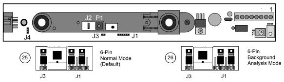
Newer Models - 3 Pin Jumper - Shown with same orientation as 6-pin jumper above
