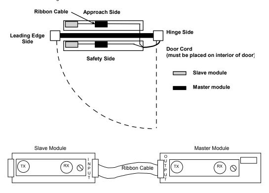
2. The angle of each module may be set independently. Use the charts below to help determine the angling. The angles may have to be altered once the units have been powered up and walk-tested.
