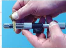
Place key in micrometer...
