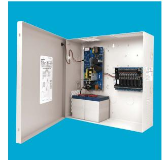
The Securitron AQD6 Series of switching power supplies are dual voltage, UL listed, supervised units. These units are field selectable with a dedicated battery charging circuit. They provide 6 Amps at 12VDC or 24VDC continuous, with up to 16 independently controlled power limited outputs.
