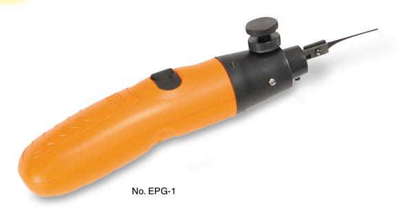
The Electropick™ was the first electric pick gun manufactured in the USA, and is still the best. The amount of "bounce" in the pick blade is adjustable, allowing you to modify the action for different locks. It comes complete with 2 straight pick blades, 2 angled pick blades, 1 medium tension wrench, and 1 rigid tension wrench.
